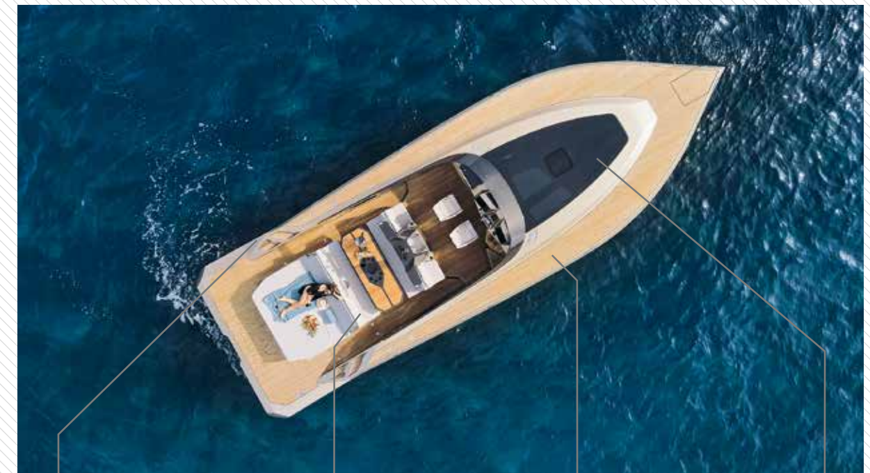
PLATFORM WINGS The fixed platform wraps around the topsides to add protection when berthing
